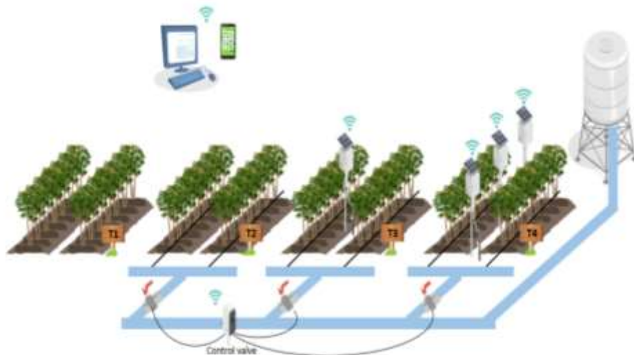
Figure 1 Diagram of irrigation treatment and wireless sensor network installation
